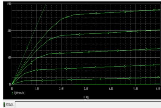
Fig-6: Simulation graph for Typ. Output characteristics
