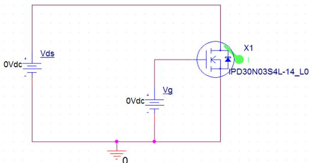
Fig-5: Circuit diagram for typ. Output characteristics
