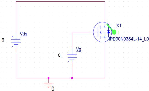
Fig-8: Circuit diagram for typ. Transfer characteristics
