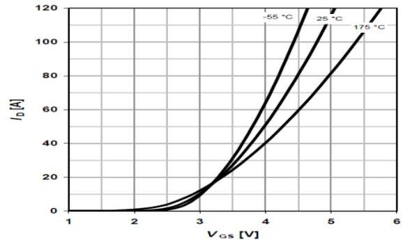
Fig-7: Typical Transfer characteristics
