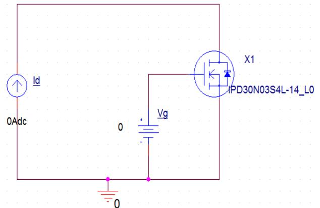
Fig-11: Circuit diagram for  $I_D$  Vs  $R_{DS(ON)}$
