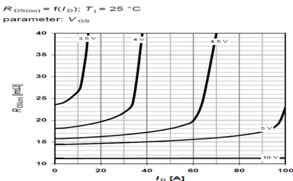
Fig-10:  $I_D$  Vs  $R_{DS(ON)}$  graph
