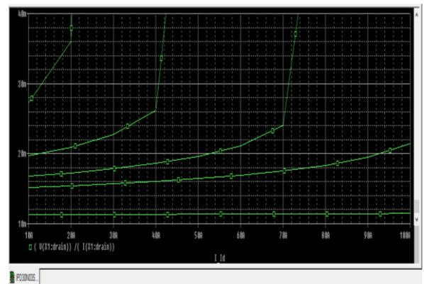
Fig-12: Simulation graph for  $I_D$  Vs  $R_{DS(ON)}$
