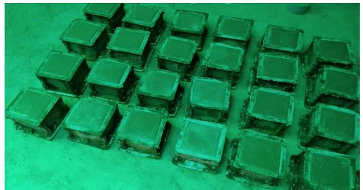
Fig. 2: - Concrete Cubes ready for curing
