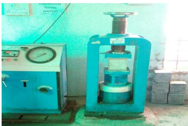
Fig.3: - Compression testing of cubes
