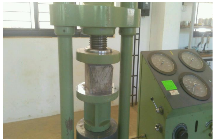
Fig -4: Test setup for cube compressive strength
