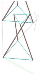
Fig -4: 3D rendering view of tensegrity tower
