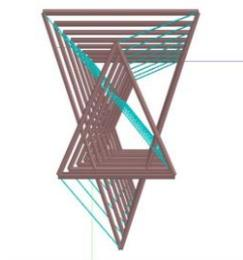
Fig -5: Projected plan of the ground surface of tensegrity tower
