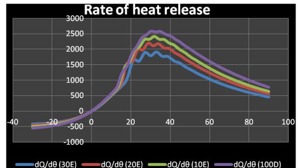
Fig 4.3 Heat Release Rate Vs Crank Angle
