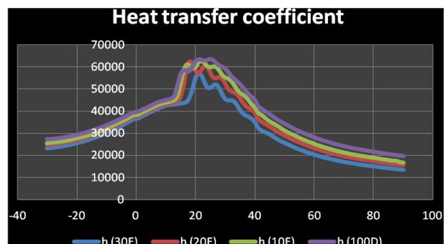
Fig 4.4 Heat Transfer coefficient Vs Crank Angle
