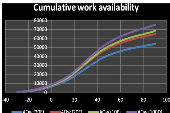
Fig 4.6 Cumulative Work Availability Vs Crank Angle
