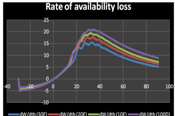
Fig 4.7 Rate of Availability Loss Vs Crank Angle
