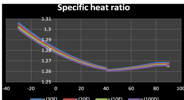
Fig 4.2 Sp. Heat ratio Vs Crank Angle
