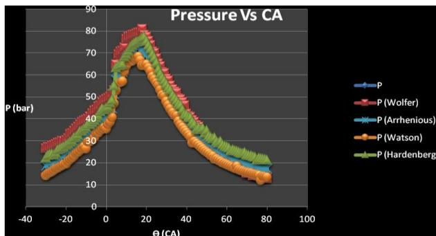
Fig 4.9 Cylinder Pressure (Predicted And Experimental) Vs Crank Angle
