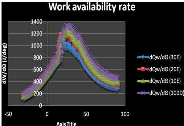
Fig 4.5 Work Availability Rate Vs Crank Angle
