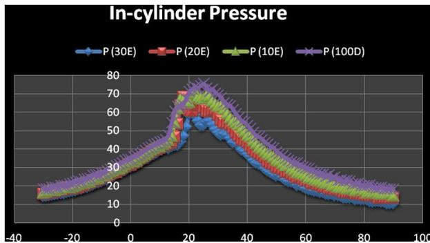
Fig 4.1 Engine cylinder pressure Vs Crank Angle
