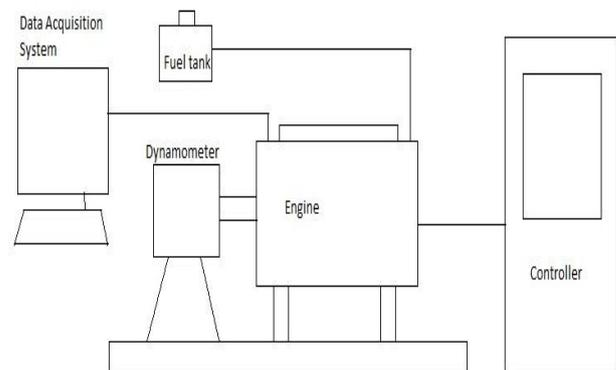
Fig. 3.1 Block diagram of Experimental setup
