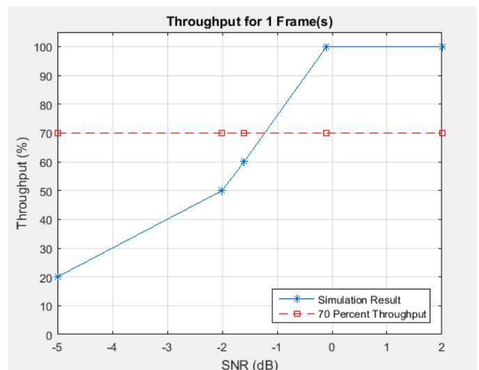
Fig-7: PUSCH Throughput against the range of SNRs of 2 Receive Antennas
