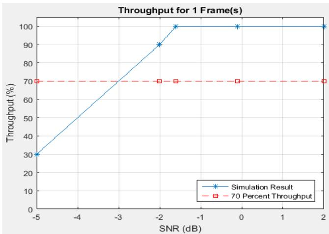
Fig-8: PUSCH Throughput against the range of SNRs of 4 Receive Antennas
