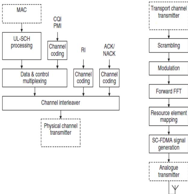
**Fig-3:** Uplink Shared Channel (UL-SCH)
