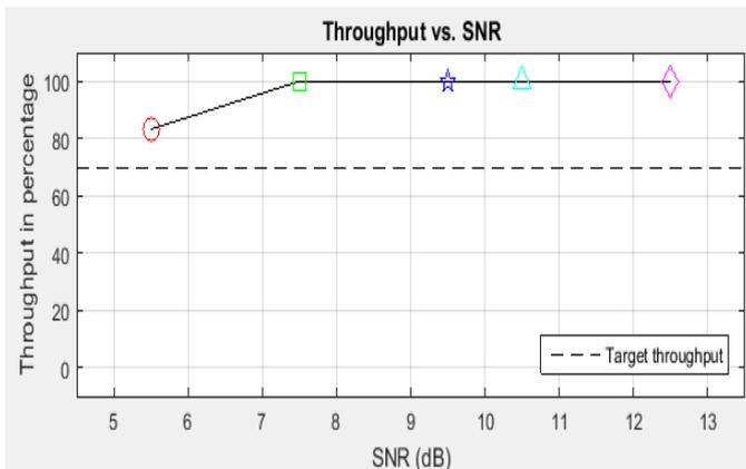
Fig-6: PDSCH Throughput against the range of SNRs for 4x4 Spatial Multiplexing
