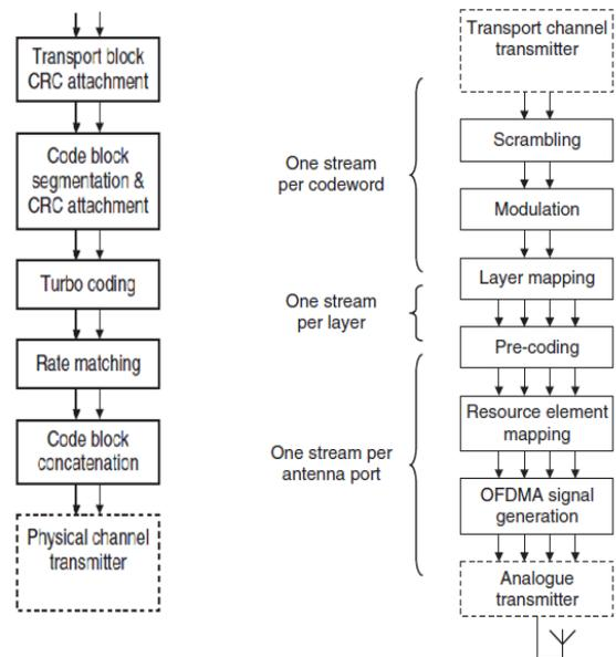
**Fig-1:** Downlink Shared Channel (DL-SCH) [7]
