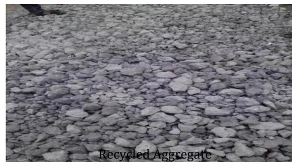
Almost all materials which are used in the construction industry were entirely natural and all waste from demolished buildings was disposed of in landfills and partially in unauthorized places. The utilization of the recycled aggregates created from processing C&DW in new construction has become more important over the last two decades.
