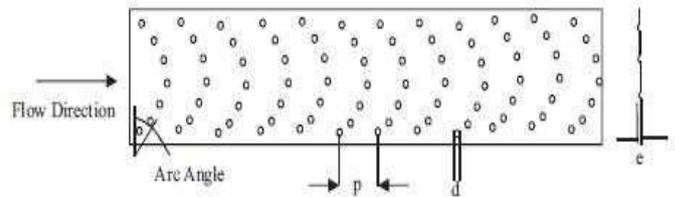
Fig. 2.12 Dimple roughness in arc manner
