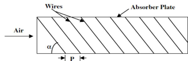
Fig. 2.2 Roughened absorber plate with inclined ribs.
