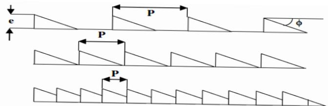
Fig. 2.7 Absorber plate having transverse wedge shaped rib roughness.
