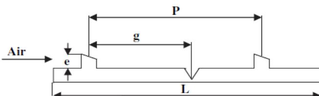
Fig. 2.9 Absorber plate having chamfered rib-grooved artificial roughness.
