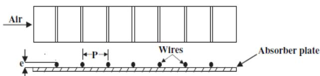
Fig. 2.1 Roughened absorber plate fixed with transverse continuous wires
