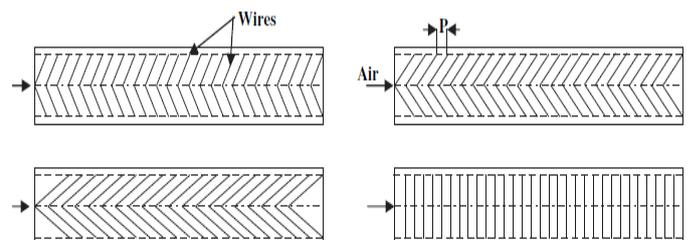
Fig. 2.3 V-shape and transverse roughness elements on absorber plate.
