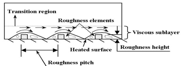
**Fig.1.** Effect of roughness elements on flow field
