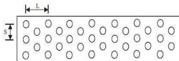
Fig. 2.11 Staggered dimple roughness
