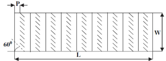
Fig. 2.6 Roughness geometry as a combination of inclined and transverse ribs.
