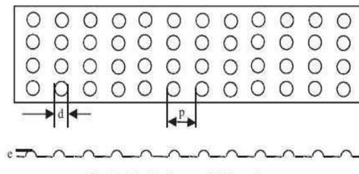
Fig. 2.10 Dimple shaped artificial roughness
