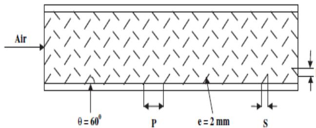
Fig. 2.4 Roughness geometry in rectangular channel as grit shape ribs Gap in an inclined continuous rib
