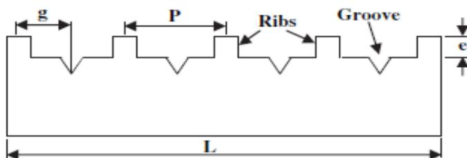
Fig. 2.8 Absorber plate having rib-grooved artificial roughness.
