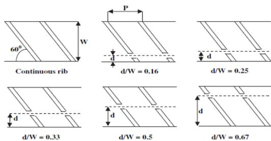
Fig. 2.5 Roughness geometry as inclined non-continuous arrangement ribs.
