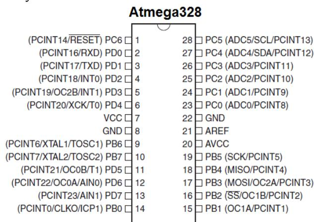
Fig 3: ATmega328 pin out
