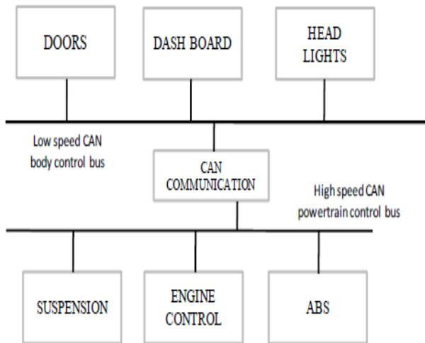
Fig 2. CAN bus system in an Automobile
