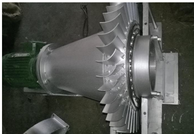
Fig -4: Experimental setup of Shaftless steam turbine
