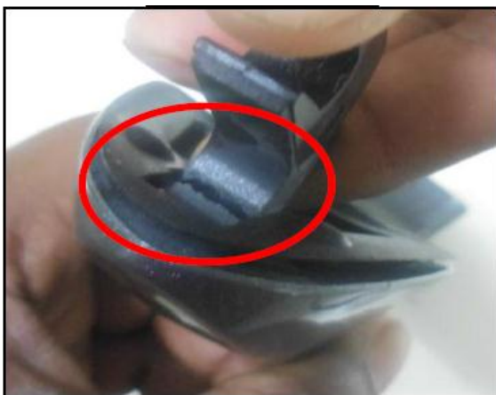
Fig. 14 Handle hinge side breakage.
