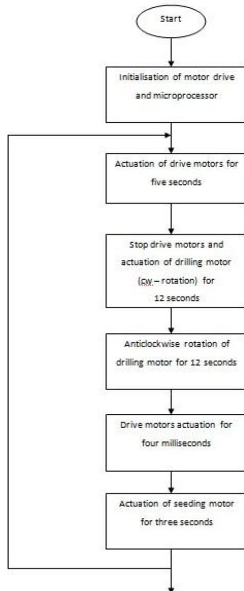
**Fig -4:** Working flowchart
