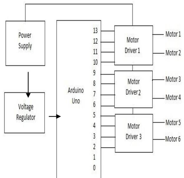
Fig -2: Block diagram of electrical assembly
