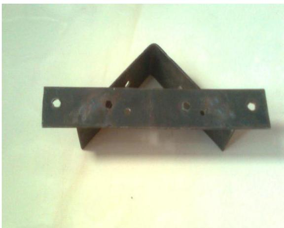
**Fig -3:** Mud closing arrangement
