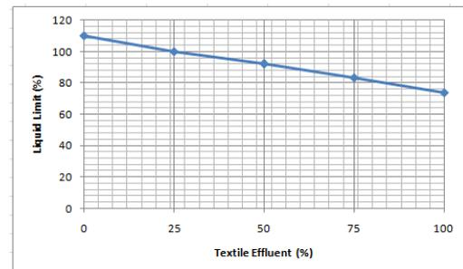
**Fig-2:** Variation in Liquid limit with varying percentages of textile effluent
