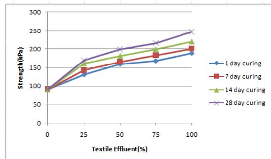
**Fig-7:** Variation of strength with varying percentages of textile effluent for different curing period
