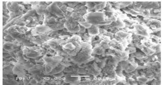
**Fig-3:** SEM image of soil mixed with 100% textile effluent
