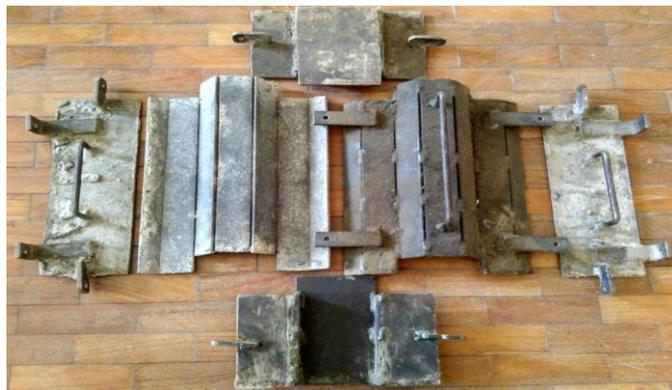
Fig -2: Parts of mould
