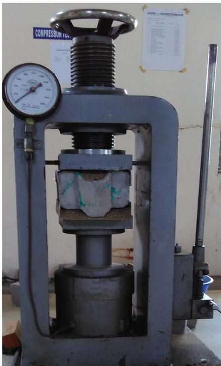
**Fig-7:** Compressive strength set up
