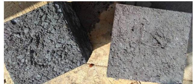
Fig -3: Cubes of M10 and M15 mix
