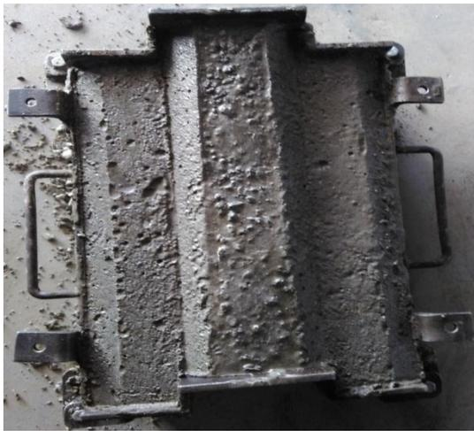
Fig -5: Interlocking block with mould
