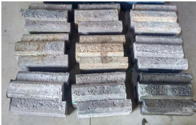
Fig -6: Interlocking blocks cast
