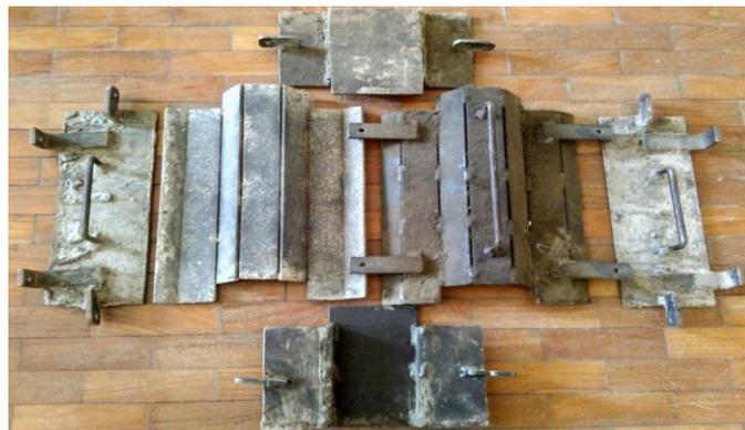
Fig -2: Parts of mould
