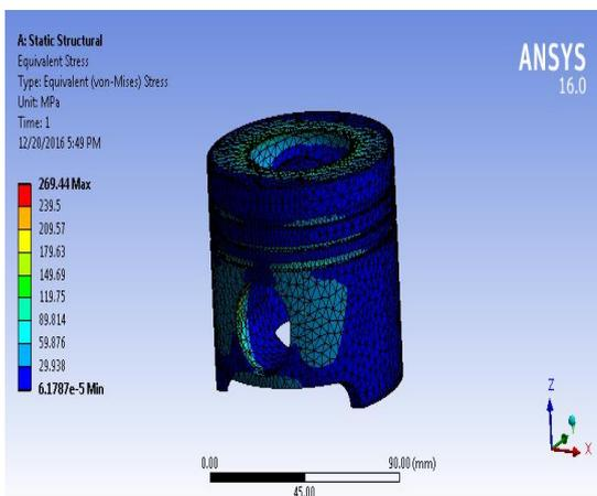
Case 4: For pressure = 5 N/mm<sup>2</sup> (For Cast Iron)
