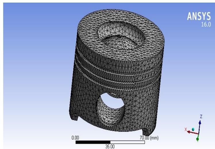
Fig 3: Meshing of Piston Model
