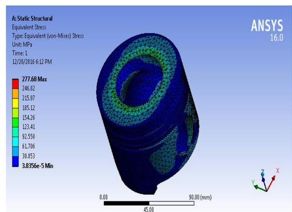
Case 5: For pressure = 10 N/mm<sup>2</sup> (For Cast Iron)
