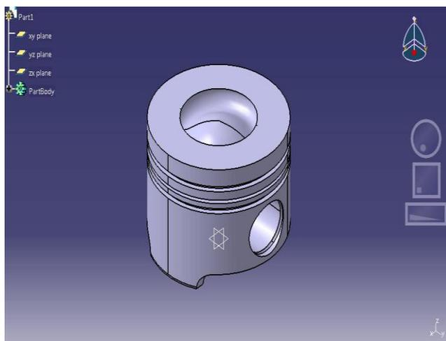
Fig 1: Piston created by CAD model
