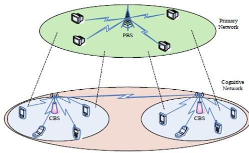
Fig-4: Structure of centralized CRN
