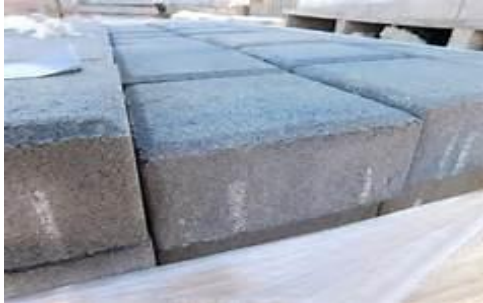
Fig -3: Marble dust Concrete Cube
