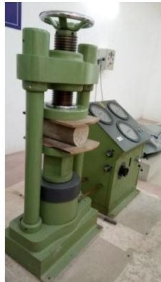
Fig-13: Split tensile strength testing machine
