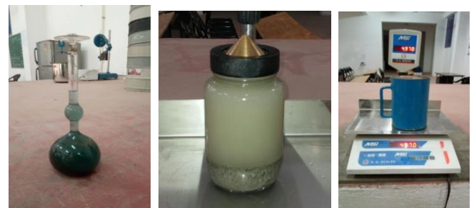
Fig-3: Specific gravity test on a) cement b) fine aggregate c) coarse aggregate
