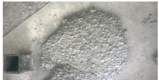
Fig.-5: Fresh Geopolymer Concrete
