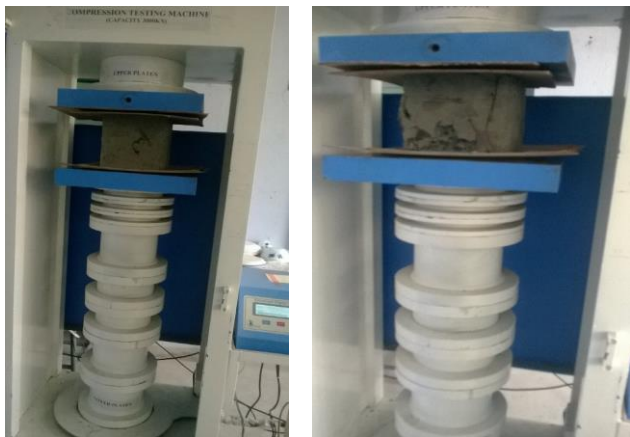
Fig.-7: Compressive Strength Testing of GPC Cubes
