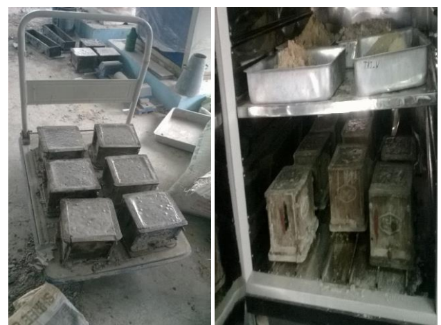
Fig.-6: Oven Curing of GPC Cubes
