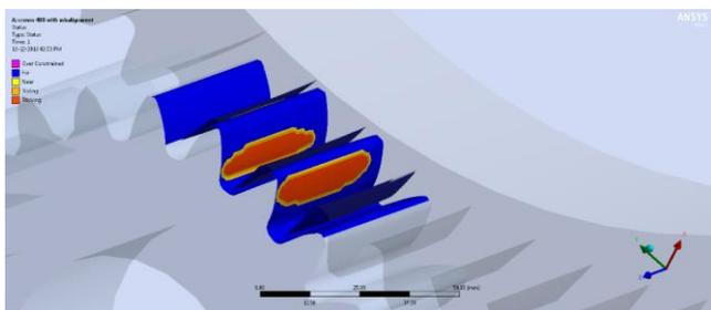
Fig. 12 Contact stress distribution (crown, misalignment)
