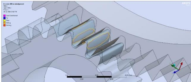
Fig. 11 Contact stress distribution (crown, no misalignment)
