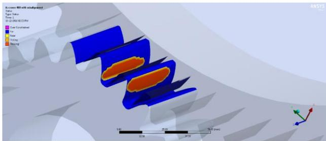
Fig. 12 Contact stress distribution (crown, misalignment)
