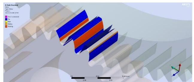
**Fig. 9** Contact stress distribution (no crown, no misalignment)
