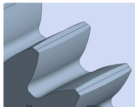
Fig. 1 Spur gear tooth with crowned teeth profile
