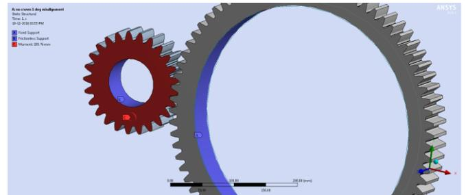
**Fig. 8** Gear pair with applied load and boundary conditions
