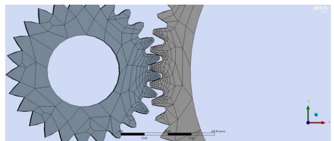
**Fig. 3** Gear mesh refined around region of contact
