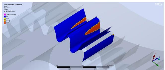
**Fig. 10** Contact stress distribution (no crown, misalignment)
