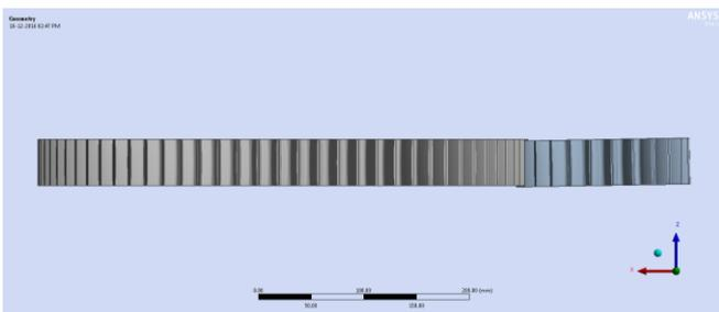
**Fig. 7** Showing crowned gear pair with misalignment
