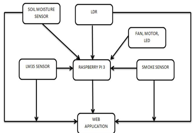
Fig -1: Block Diagram of Smart Agriculture Management System
