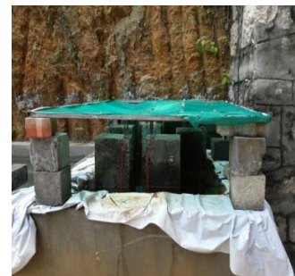
Fig – 3: Accelerated corrosion technique set up
