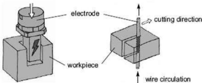
Fig.-2: Die sinking & wire cut EDM Process
