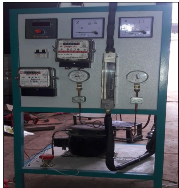
Figure 3.2: Actual Test Setup of VCRS with Nano Refrigerant
