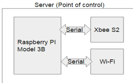
The smartphone/web client uses JSON objects and REST API implemented in the server to communicate bidirectionally with the server, the server abstracts the ZigBee interface layer, uses a simple datagram to deliver information to the respective ZigBee device after which the paired Arduino will do the respective action. Use of REST API allows any device to communicate with server thus making it flexible.
