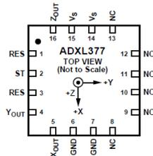
Fig -4: Pin configuration of ADXL377 [3]
