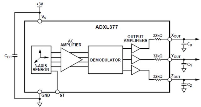
Fig -5: Functional block diagram of ADXL377 [3]
