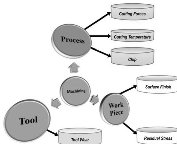
Fig. 1. Main factors to consider when working with hard turning
