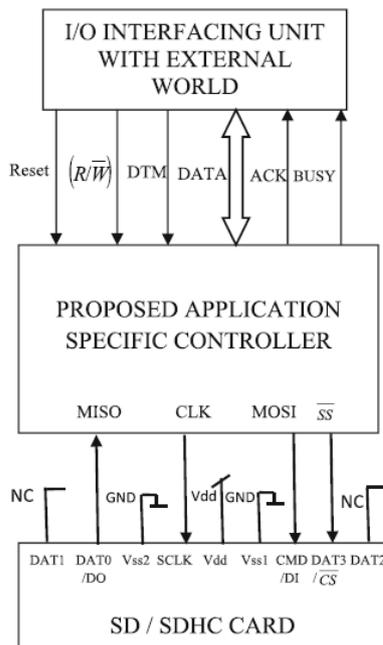
Fig. 4 Overall schematic of the proposed controller
