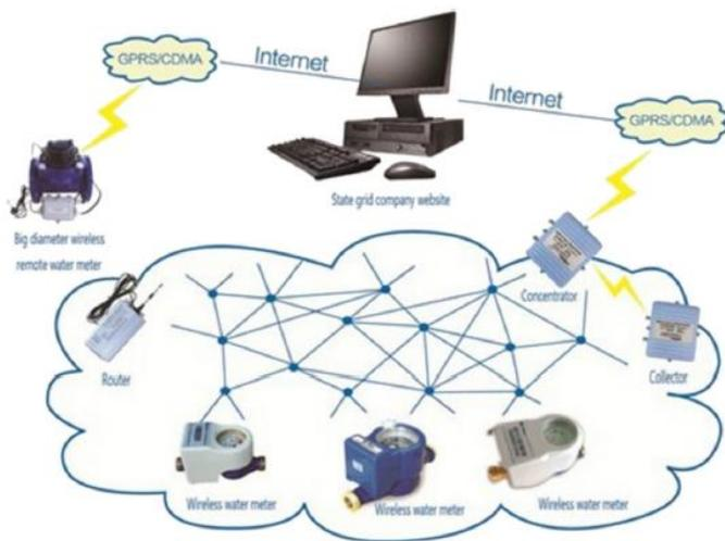
**Fig. 2** Block diagram of a real-time data concentrator system
