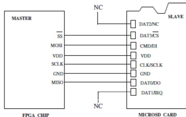
**Fig. 3** Micro Secure Digital (SD) card electrical interface with FPGA board
