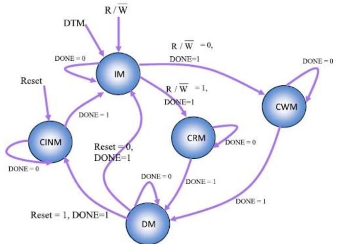
Fig. 5 State diagram of the controller
