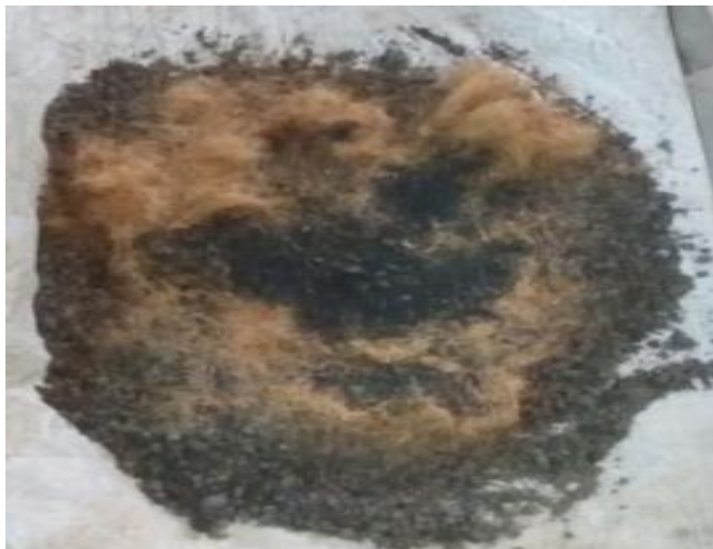
Fig -1: Mix of pond ash, coir fiber, copper slag and clay
