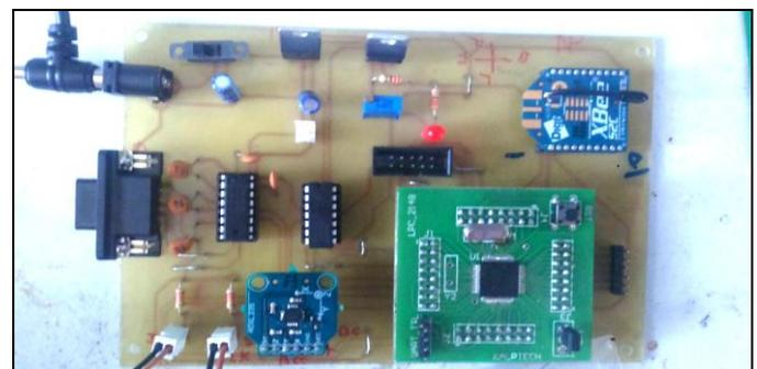
Figure 3. Transmitter Prototype
