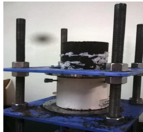
Fig -3: Plastic Strips with Soil
