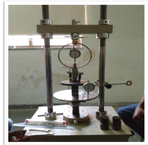
Fig -4: UCS Testing Machine
