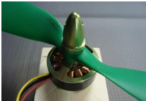
Fig.3. Higher KV BLDC motor with Small propeller Combination [8]
