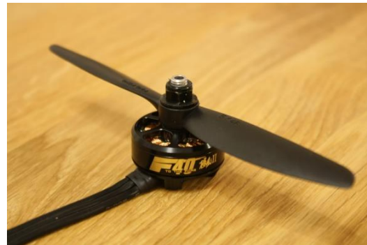
Fig.4. Less KV BLDC motor with higher propeller combination [9]
