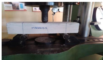
Fig -5: Flexural failure of M302D0.5
