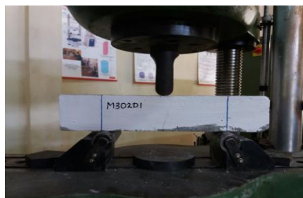
Fig -7: Flexural failure of M302D1
