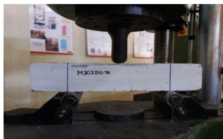
Fig -6: Flexural failure of M302D0.75
