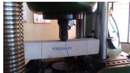
Fig -4: Flexural failure of M302D0.25
