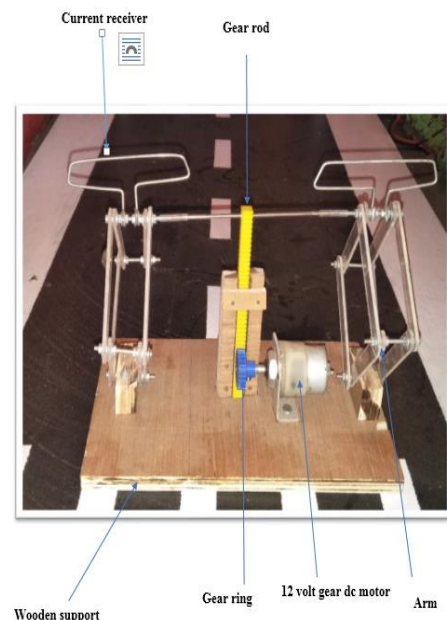
Fig -3.5 concept pantograph module
