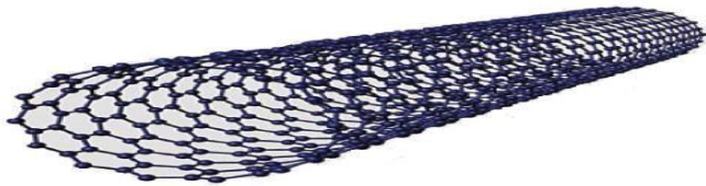
Fig-8: Rolled up sheet of graphene.
