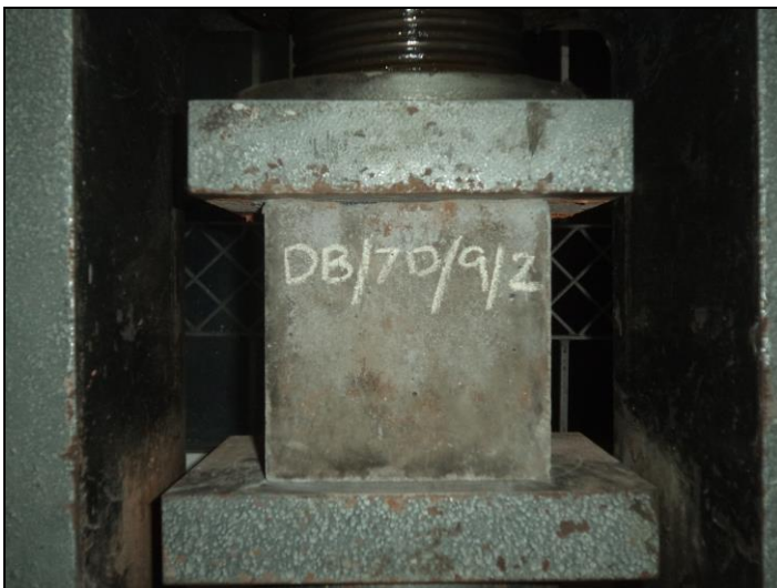
FIG.2. Test for Compressive strength of Concrete
