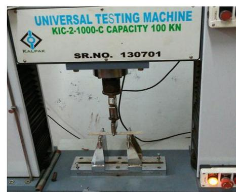
**Fig -2: Flexure Test**
