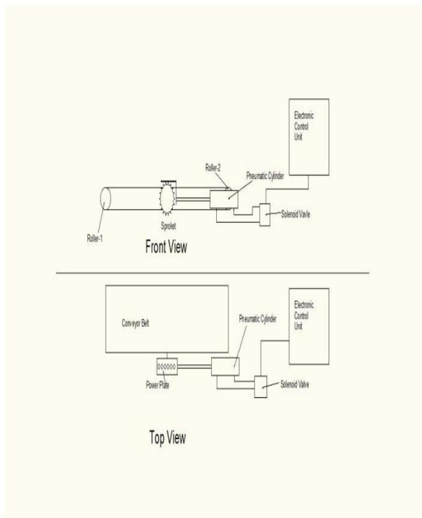
Fig- 1: Block Diagram of Project
