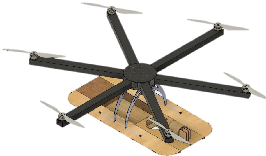
Figure 1 – 3D Design of AAUAV (Hovercraft plus Multicopter)
