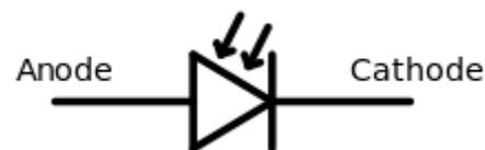
Figure 6: Symbol of a Photodiode
