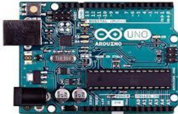
Fig -3: Arduino Uno Board
