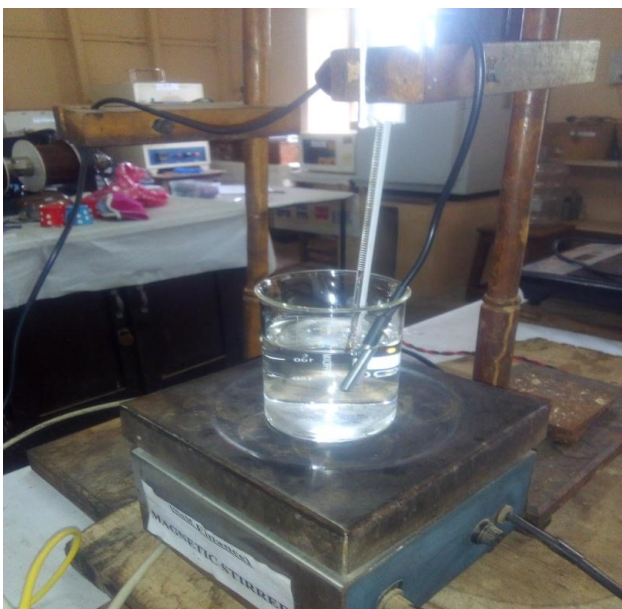
Fig-4?: DS18B20 is inside the water system. An additional thermometer is for calculating the accuracy of the experiment
