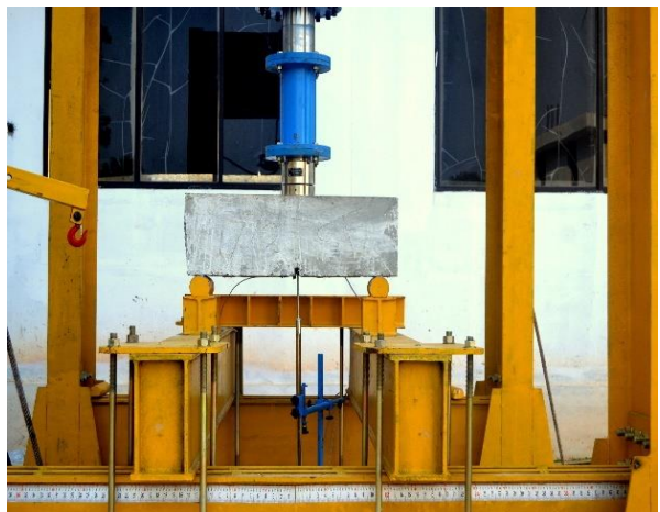
Fig 14 Fracture test set up of notched steel
