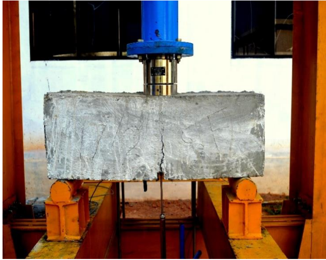
Fig 15 Crack appearing on notched steel fiber reinforced concrete beam
