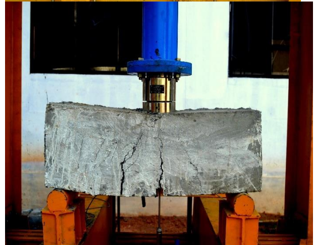
Fig 12 Fracture test set up of notched beam
