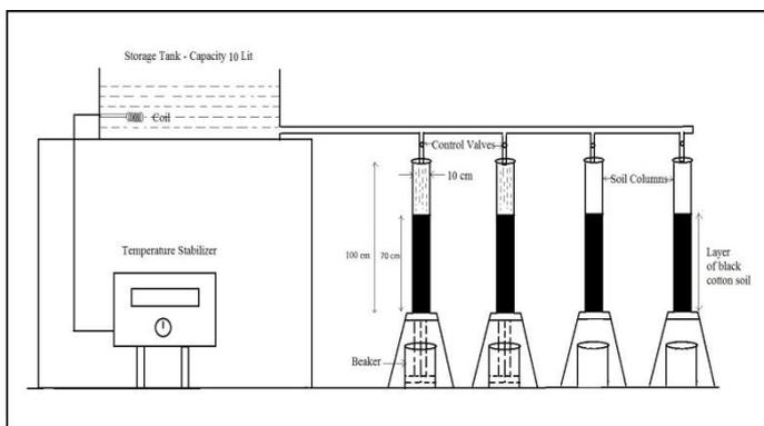
Fig 2- Proposed Setup of Soil Column Simulation of SAT Process
