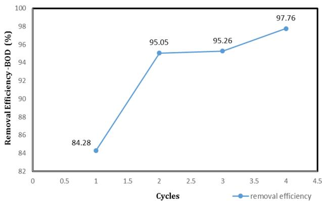
**Chart - 1 :** Graphical representation of cycles Vs. removal efficiency BOD
