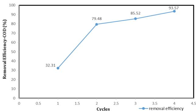
**Chart - 2 :** Graphical representation of cycles Vs. removal efficiency COD
