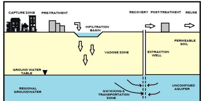
Fig 1- Layout depicting various Components of SAT
