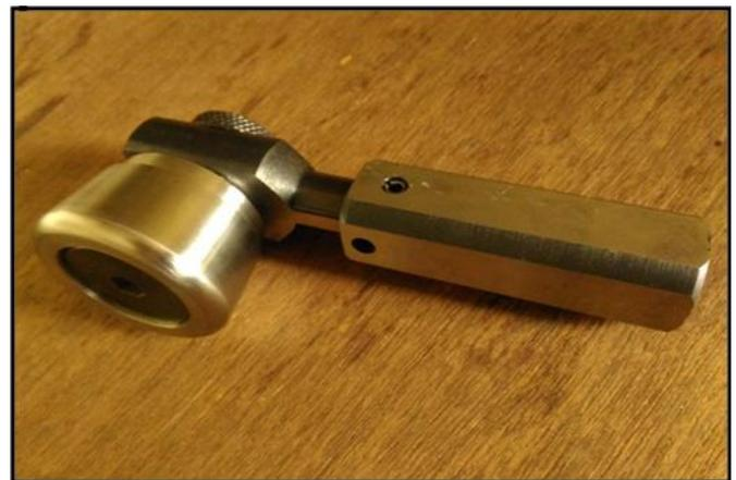
Fig -2: Single Roller Burnishing Tool
