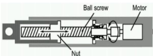
Fig.2 Ball screw harvester
