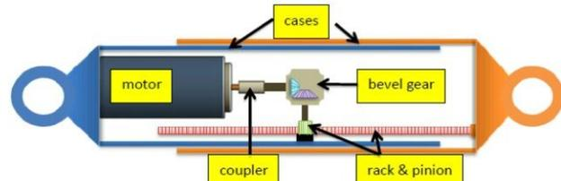
Fig.3 Rack-pinion electromagnetic damper
