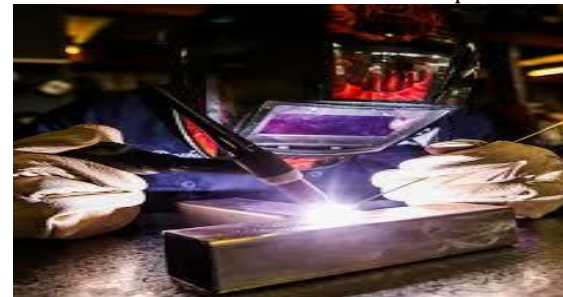
Figure 3.4: Welding of EN8 steel
