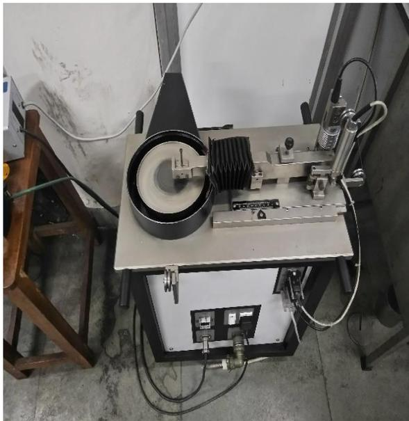
Fig -1: Pin-on-disk tribometer
