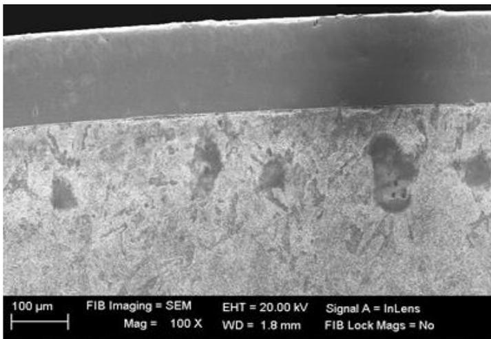
Fig-6 SEM image of coated plate
