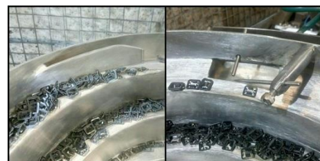
Fig-3: Wiper Blade and Needle Tools
