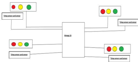
Figure 2: Block diagram of traffic control system
