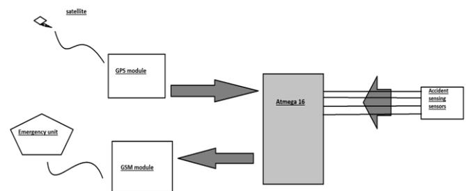
Figure 1: Block diagram of Accident Alerting Mechanism
